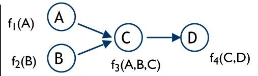
**Step 1 (Restriction):** Replace  $f_4(C,D)$  with  $f_5(C) = f_4(C,d)$
