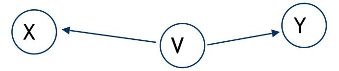
There exists a variable *V* on the path such that it **is** in the evidence set *E* the arcs putting *V* in the path are "tail-to-tail" Or, there exists a variable *V* on the path such that it **is** in the evidence set *E* the arcs putting *V* in the path are "tail-to-head"
