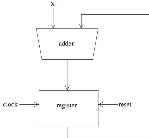
“Clock” and “reset” each correspond to one input switch. “X” is four input switches, constituting a four-bit binary number.
